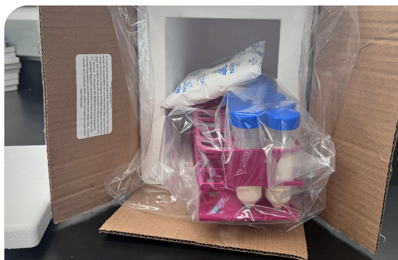
The labeled milk samples were placed in a rack and then bagged prior to shipping in a cooler with packing material and cooling packs.
