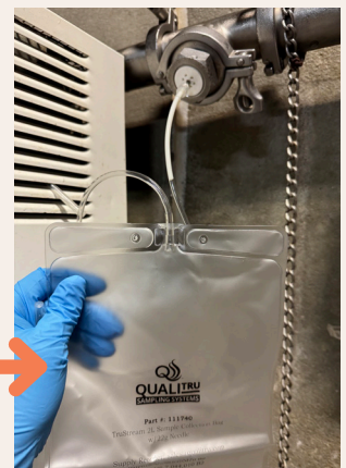
Milk sample being collected using a needle inserted into a septum in the pipeline. The milk travels through tubing that leads to a bag kept in the refrigerator.
