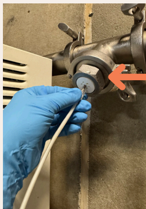
Milk sample being collected using a needle inserted into a septum in the pipeline. The milk travels through tubing that leads to a bag kept in the refrigerator.
