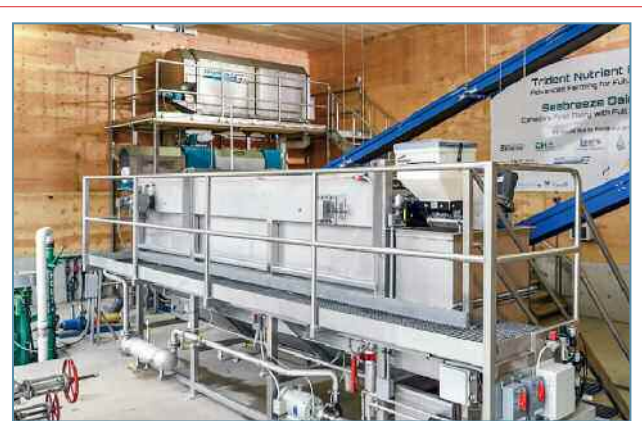
A Trident nutrient recovery system.
