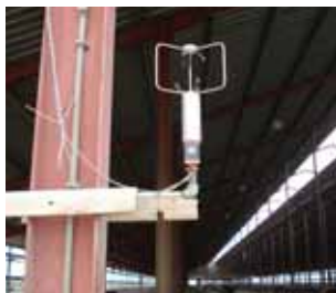
Air emissions monitoring equipment gathers data from inside a dairy barn.
